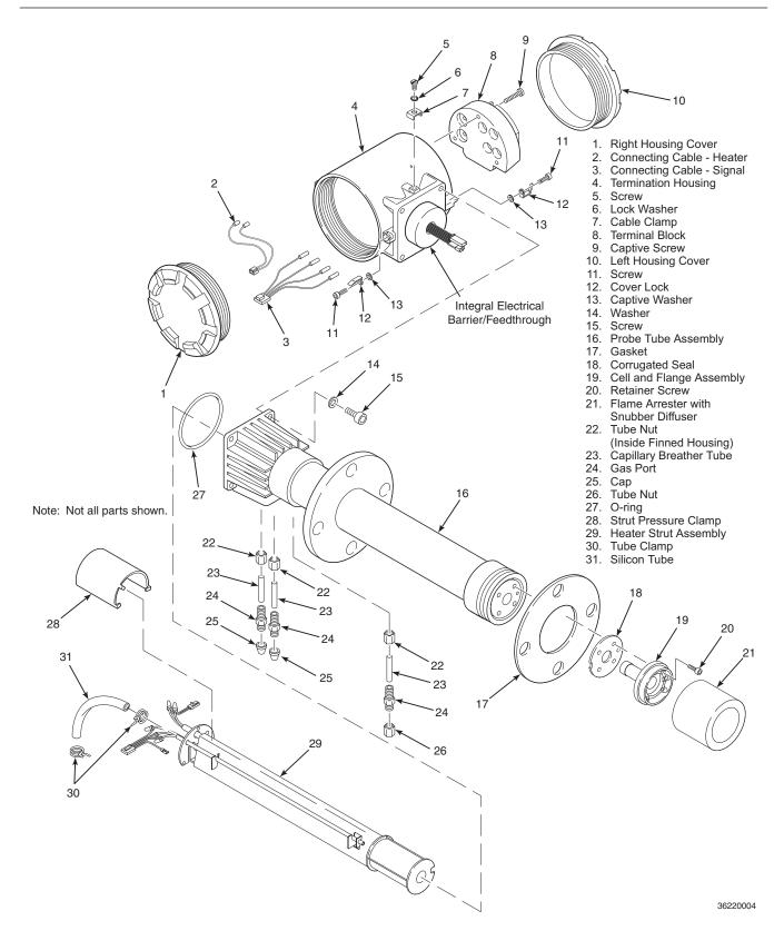
Figure 4-1. Hazardous Area Oxymitter DR Exploded View
